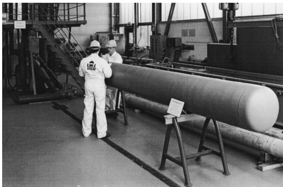
Fig. 2. Hydrogen storage in metal hydride cylinders.
