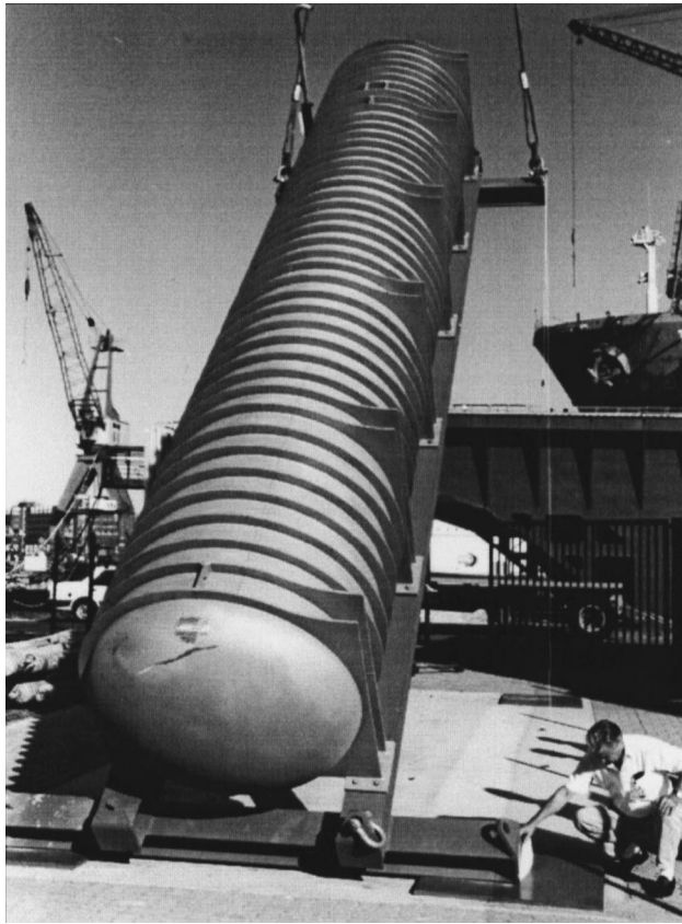
Fig. 4. Liquid oxygen storage tank.
